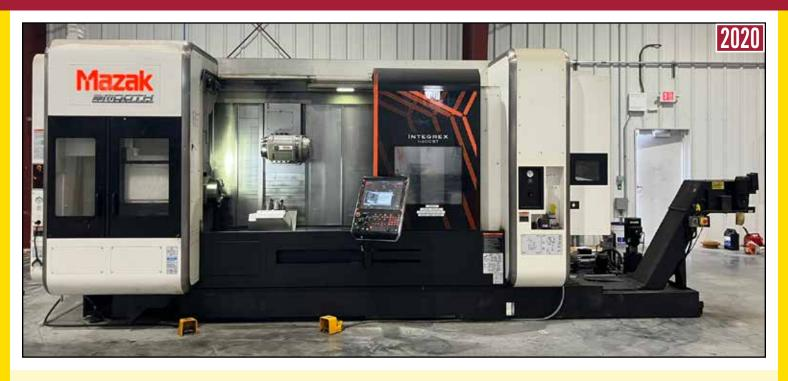
MAZAK INTEGREX i400ST/1500U 5-Axis Multi-Tasking CNC Lathe with Second Spindle & B-Axis Milling, 12" 3-Jaw Hydraulic Chuck (Main), & 10" 3-Jaw Hydraulic Chuck (Second), 59.8"Machining Length, Main Spindle Speeds to 3,500 RPM, Second Spindle Speeds to 4,000 RPM, B-Axis Spindle
