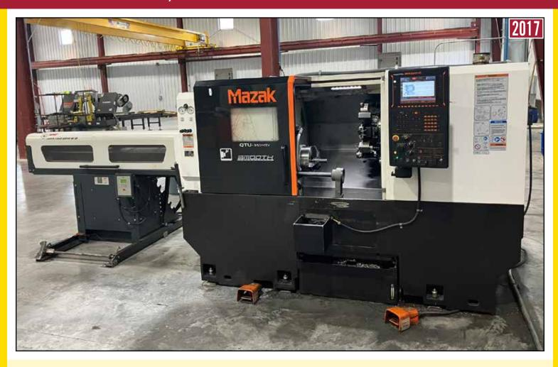
MAZAK QUICK TURN Universal 350MSY CNC Lathe with Sub Spindle, Y-Axis & Live Milling, 10" 3-Jaw Hydraulic Chuck (Main) & 8" 3-Jaw Hydraulic Chuck (Sub), 27.4" Swing x 27" Center Distance, 3.2" Bar Capacity, Spindle Speeds to 3,500 RPM (Main/Sub), Y-Axis Spindle Speeds to 6,000 RPM, 12 Position Turret, TSC, Tool Presetter, Auto Parts Catcher, Chip Conveyor, LNS Quick Load Servo 80 S2 Barfeed, MAZATROL Smooth C CNC Control, sn:280063, mfg.2017 (Cons #1)
