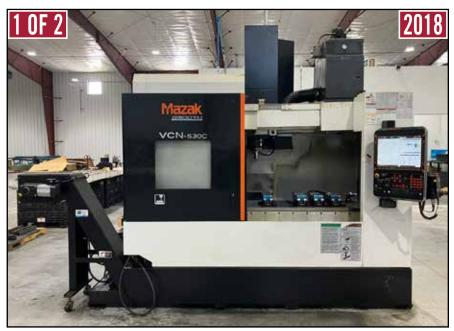
(2) MAZAK VCN-530C CNC Vertical Machining Centers with 51.2" x 21.6" Tables, #40 Spindle Speeds to 15,000 RPM, Approx. 41.3" X-Axis Travel, 20" Y-Axis, 20" Z-Axis, 48 Position ATC, HPTSC, Chip Conveyor, RENISHAW Dual Probe, MAZATROL SmoothG CNC Control, sn:296520, mfg.2018 (Cons #1), sn:280079, mfg.2017 (Cons #1)
