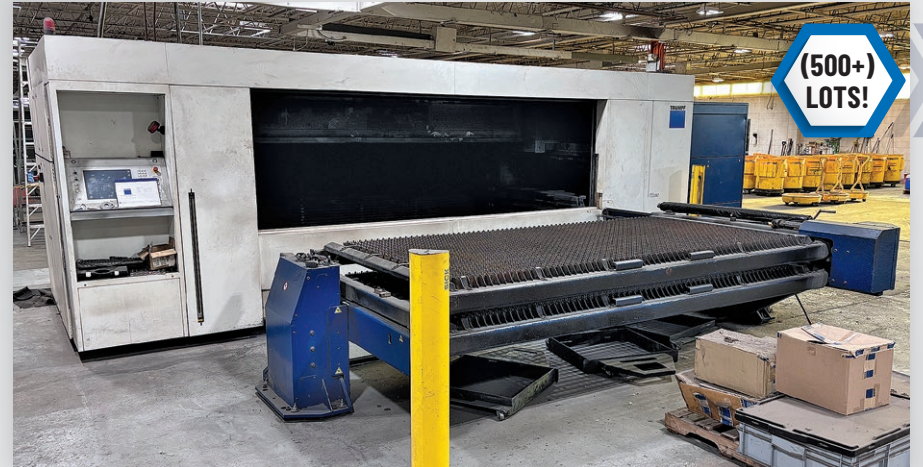
2,000 Watt Trumpf Model Tru-Laser 1030 CNC Fiber Laser
