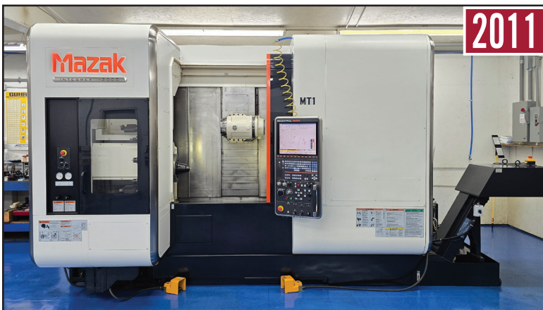
2011 MAZAK Integrex i-200S Horizontal Machining Center, sn 225580, Twin Turning Spindles, True 5-Axis Capacity, 40-Station ATC, 8" Collet Chuck, Mazatrol Matrix DRO Control
