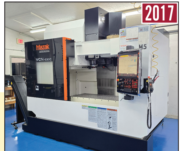
2017 MAZAK VCN-530C Vertical CNC Machining Center, sn 279878, MAZATROL SmoothG DRO Control, 51" x 21 1/2" Table, Set Up for NIKKEN CNC260 4th Axis, 15,000 min-1 Max Spindle Speed, 30-Station ATC, CAT-40 Taper, Outfeed Chip Conveyor
